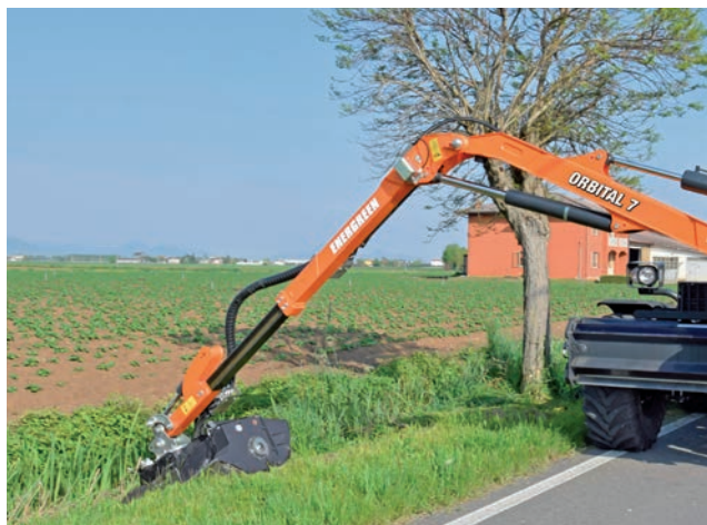
104 Decespugliatori semoventi, macchine per operazioni heavy duty Self-propelled brush cutters, machines for heavy duty operations Pietro Piccarolo
